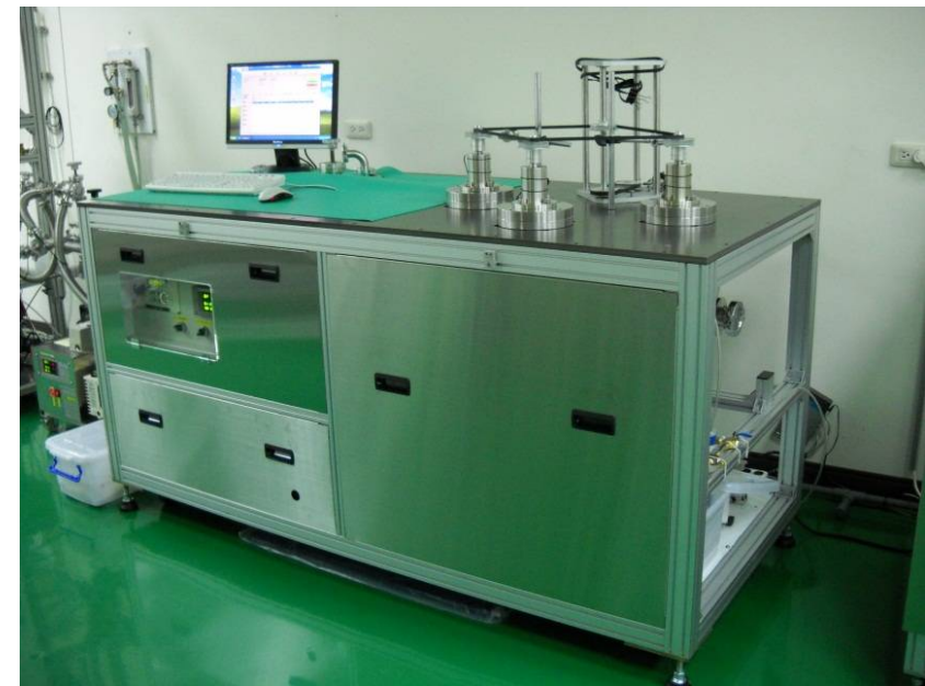
Feedthrough dynamic process testing
